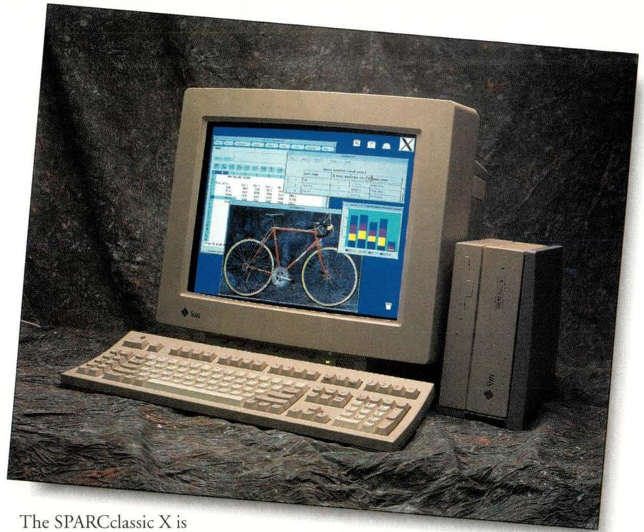
The SPARCclassic X is based on the microSPARC, operating at 50 MHz. It comes with 4 to 96 MB of main memory and 6 KB of cache and supports 8-bit color. The product offers 1.54 to 2.33 Xmark scores, and 29,900 to 102,600 Xstones. The terminal's pricing starts at \$2,445 with 4 MB of memory and a 14-inch color screen, or \$2,395 each for a dozen.
