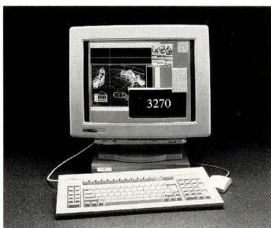
minals that support local 3270 terminal emulation and directly connect to mainframe systems. Called the HDS ViewStation TR Series, the machines can have up to four IP addresses (one for each network) and can act as a network router. In addition to the support for 3270 emulation, the machines also have a variety of local X clients, including VT320 emulation, a PostScript display application, a clock, calculators and screen savers.
