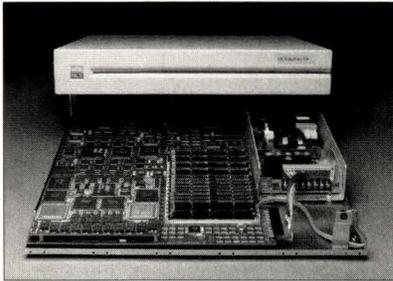
with up to eight Intel Corp. 80860 (i860) processors. The company says a Model 40 SPARCstation with one such board could have an aggregate performance of 662 MFLOPS on numerically demanding tasks. A Model 514 SPARCstation with such a board, meanwhile, would have an aggregate performance of 746 MFLOPS.
