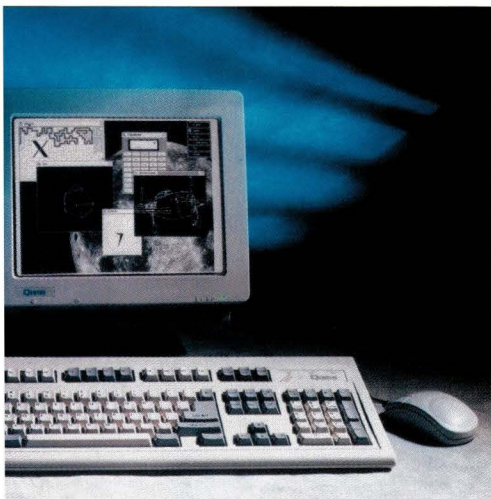
Double duty: The Qume QX15 can act as a VT220 or an X terminal.
