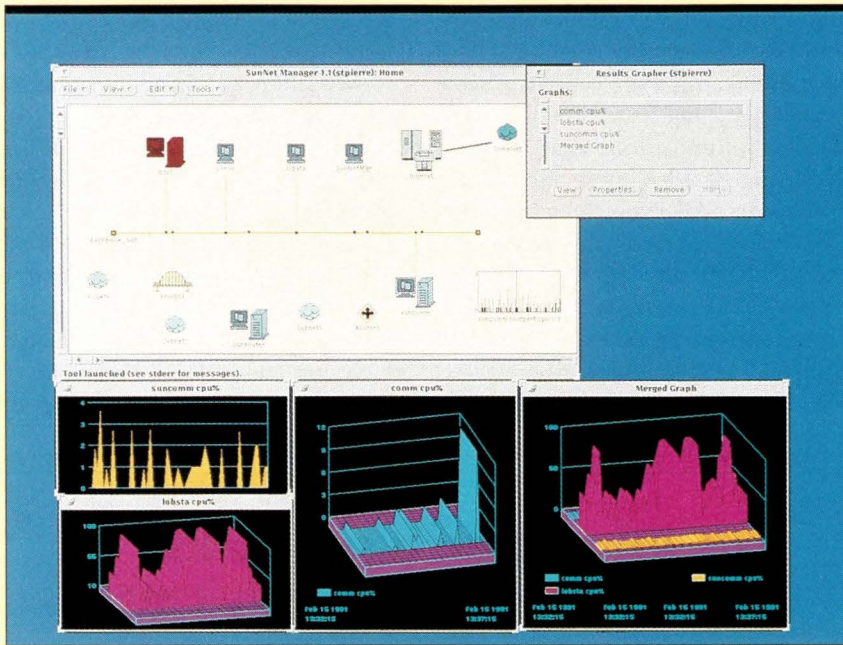
SunConnect's SunNet Manager 1.2 offers users the ability to take data from multiple inputs and graph the values over time using "Results Grapher."
