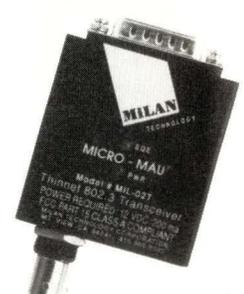
MILAN Technology is a leading designer and supplier of micro-sized Ethernet LAN products for the workstation market. The company's transceivers, converters and multiports provide the smallest, most efficient and cost-effective networking solutions in the industry.
