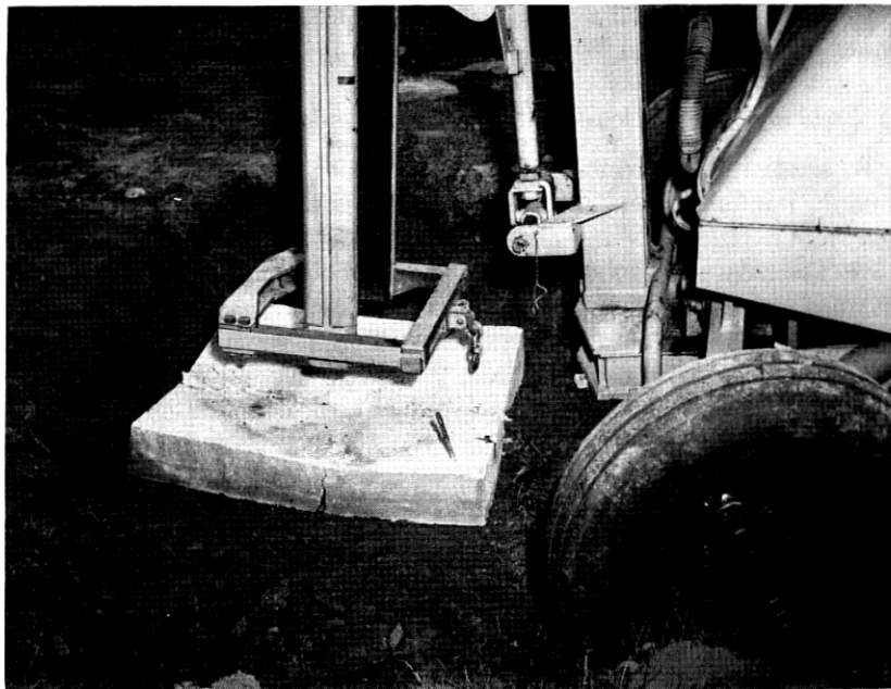
Fig. 5 — Reinforced concrete slab after one blow of 6750 foot-pounds.
