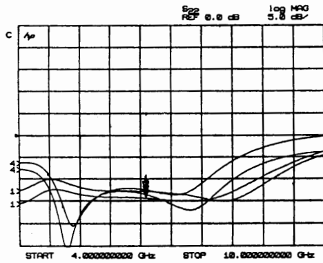
Figure 2c. Simulated return loss vs frequency for the ratrace coupler.
