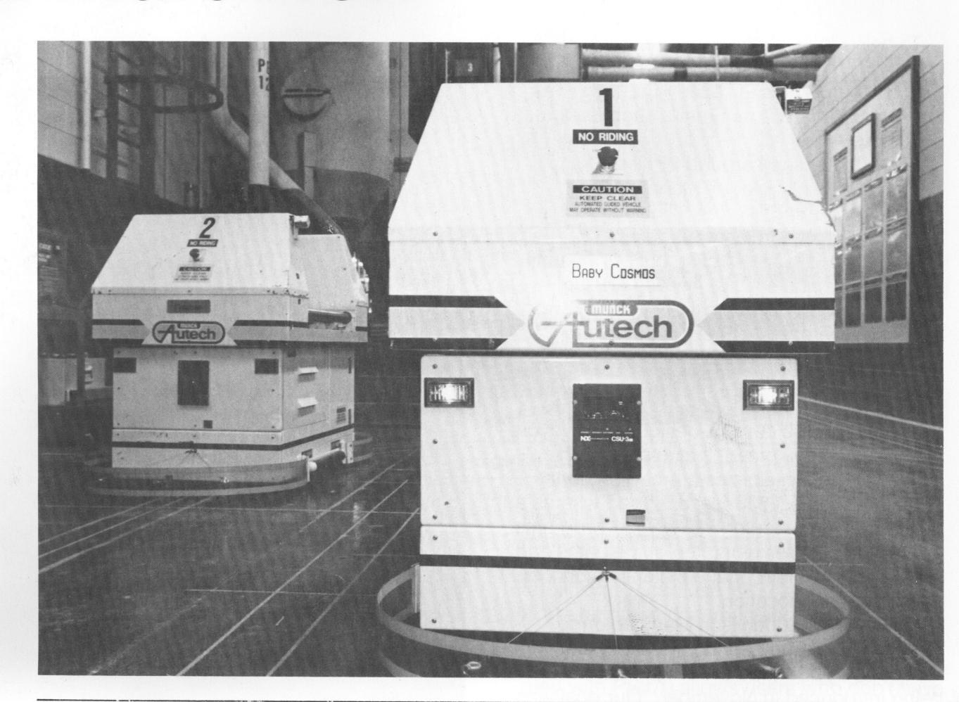
Baby Cosmos (right) and Marathon stand ready to move assembly components from one work area to another. These units are GTE's first Automatic Guided Vehicles to serve printed circuit board fabrication and fine-line departments.
