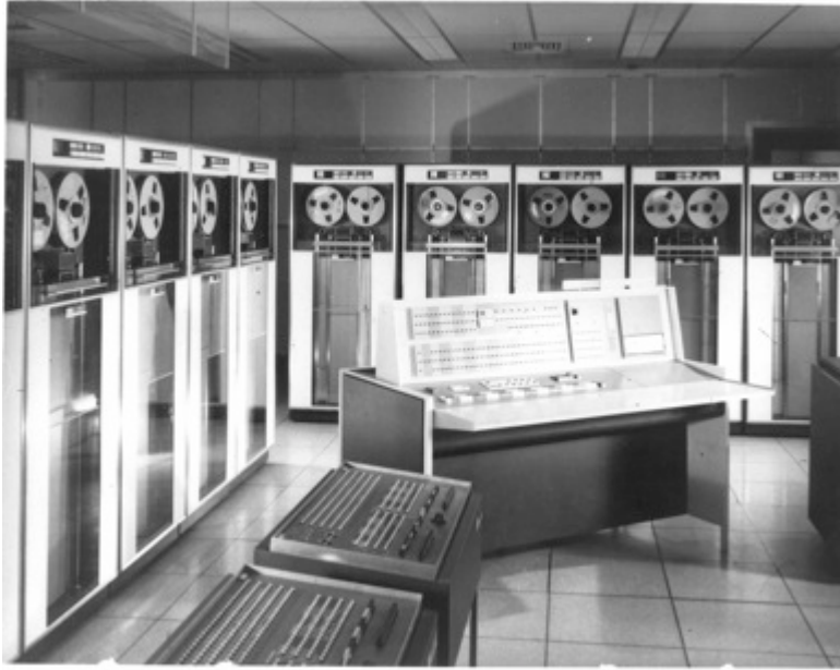
Fig. 3-1. The computer center at Bell Labs in Murray Hill around 1963 consisted of an IBM 7090 computer. Input and output were on magnetic tape. The operator monitored the operation of the computer at a console. [Photo courtesy of Alcatel-Lucent USA Inc. / Bell Labs.]
