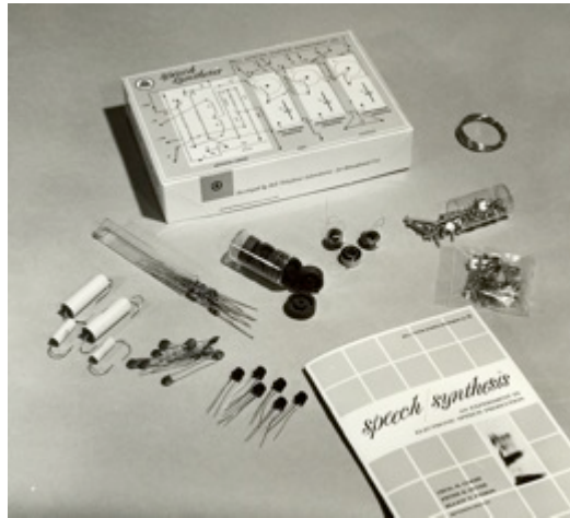
Fig. 3-8. Bell Labs created kits to demonstrate scientific principles to high-school students and distributed these kits for free. One kit demonstrated the basic principle of speech synthesis. [Courtesy of the AT&T Archives and History Center.]
