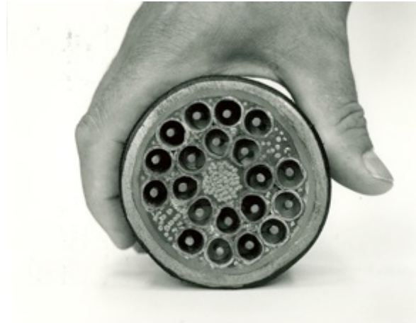
Fig. 5-11. Ten pairs of coaxial pipes formed a single cable in the L4 carrier system, first placed in service in 1967. The cable was buried underground with repeater amplifiers every 2 miles. [1965 photo courtesy of Alcatel-Lucent USA Inc. / Bell Labs.]
