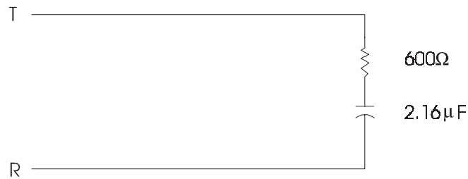
Figure 8-3. 600-Ω Quiet Termination
