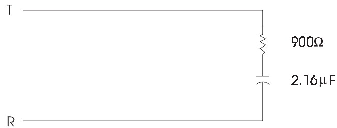
Figure 8-2. 900-Ω Quiet Termination
