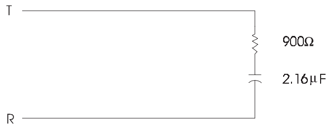
Figure 8-2. 900-Ω Quiet Termination
