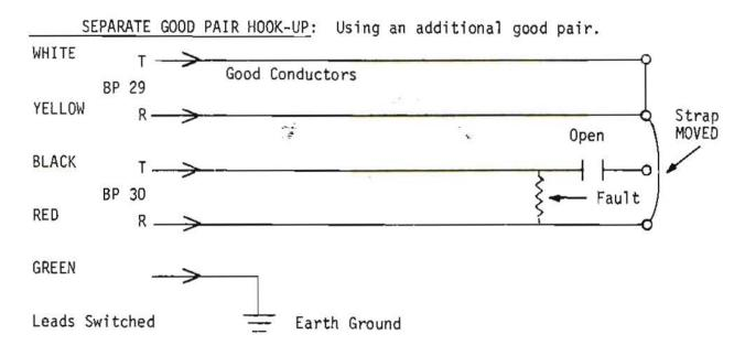
Strap is moved to the conductor that is not open - red and black leads are switched.
