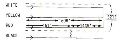
LOOP LENGTH- THE TOTAL CONDUCTOR LENGTH FROM THE WHITE TEST LEAD TO THE RED TEST LEAD. (+) or (-) 1% of digital dial reading.
