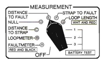
THE SET READS THE RESISTANCE (LENGTH) OF THE CONDUCTOR CONNECTED TO THE RED LEAD. THE DISTANCE TO FAULT IS THE LENGTH OF WIRE FROM THE SET TO FAULT.
