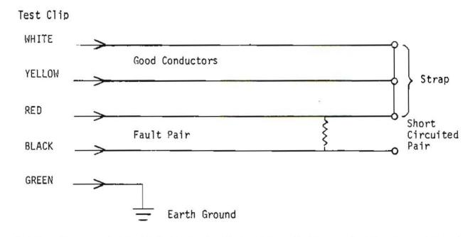
Red lead to fault and Black lead to other conductor involved in fault.
