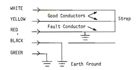
SEPARATE GOOD PAIR HOOK-UP: Using an additional good pair.
