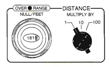
MULTIPLY THE DIAL READING BY THE SETTING OF THE "MULTIPLY BY" KEY .....
