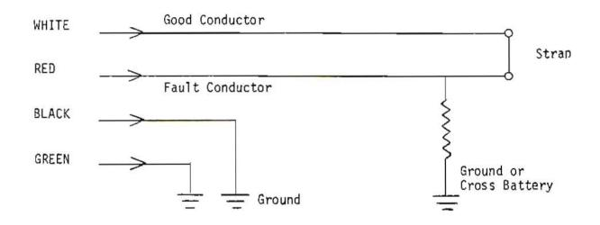
$\underline{\text{Black}}$  lead connected to ground when faulted conductor touches ground or battery.
