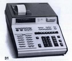
35 Built-in Math Function Keys 25 User-Definable Function Keys Complete Alphanumeric Keyboard Optional Silent Alphanumeric Printer
