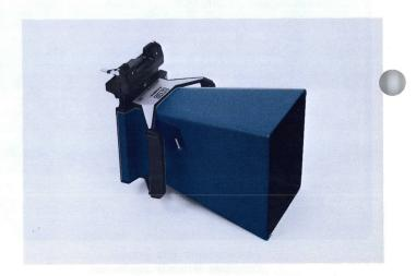
**Camera**—The C-10 is a fixed-focus, light-weight camera designed for use with all Tektronix Information Display Products which have an 11-inch CRT. An f/8 lens with sufficient depth of field and convenient hand grips allows the C-10 to be held against the display area for photographing displays. The C-10 includes a Polaroid<sup>1</sup>  $4 \times 5$  film holder.
