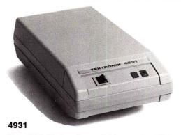
The 4931 Modem is available as an option installed internally in 4010 Family terminals or in stand alone form as pictured above. These Bell compatible Modems are available in 300 baud full duplex, 1200 baud half duplex, and 1200 baud half duplex with supervisor channel. All are designed to work on unconditioned voice grade phone lines with a DAA (Direct Access Arrangement).
