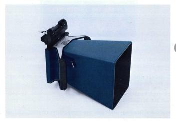
Camera—The C-10 is a fixed-focus, light-weight camera designed for use with the Type T4005. An f/8 lens with sufficient depth of field and convenient hand grips allow the C-10 to be held against the display area for photographing displays. The C-10 housing accommodates a Graflok $^1$  4 x 5 back.
