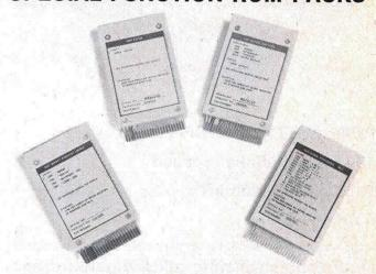
Special function ROM packs are accessories that plug into the 4051 backpack or into the 4051E01 ROM Expander Unit. The ROM packs provide additional 4051 commands, without using any read/write memory.
