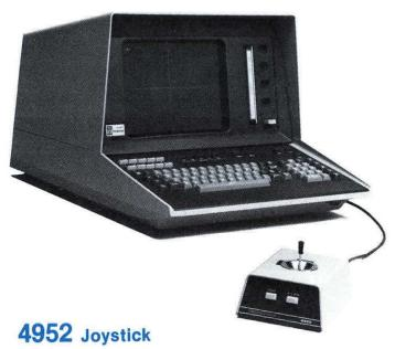
For desktop computer users needing increased interactivity, the 4952 Option 2 Joystick is the last word in fingertip input control. Accurate to 0.1%, the sensitive cursor control activated by the POINTER command lets you quickly position the cursor the first time precisely.
