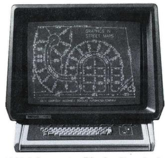
4016-1 Computer Display Terminal 25 in (63.6 cm) Direct-View Storage Display High-Resolution, Flicker-Free Graphics Selectable Formats in Graphic and Alphanumeric Modes Plug-In Intelligence Options
