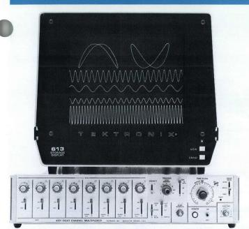
The 4701 Eight-Channel Multiplexer and the 613 Storage Display comprise a system capable of portraying eight different signal sources.
