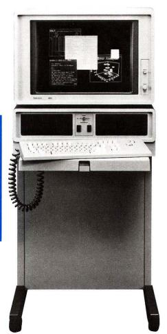
Pedestal Configuration: Display shows new 4115P51 feature enhancement which enables efficient implementation of host-based window management functions.
