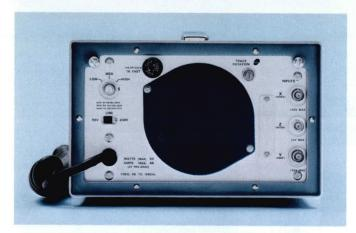
Signal input is via BNC connectors on the rear panel.
