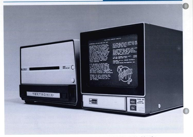
The Type 611 Storage Display Unit (MOD 162C shown) is ideally suited for information display applications. Up to 4000 alphanumeric characters may be stored and legibly displayed. These displays are directly copied by the 4601, providing an accurate representation of the display on 3M Type 777 Dry-Silver Paper.
