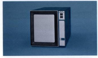
The 611 Storage Display Unit is designed to function as a readout device for computer terminals. With X, Y and Z input signals provided by peripheral equipment, this instrument is capable of displaying high-density alphanumeric and complex graphic information without drift or annoying flicker. The screen is 21 cm  $\times$  16.2 cm with resolution equivalent to 400 (vertical) and 300 (horizontal) stored line pairs. 4000 characters, 90  $\times$  70 mils in size may be clearly displayed.
