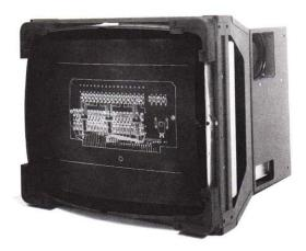
By placing fixed or finalized data in store while retaining dynamic or working data in refresh, you can work interactively with high density graphics and alphanumerics while making maximum use of processing power to address the application rather than support the display.
