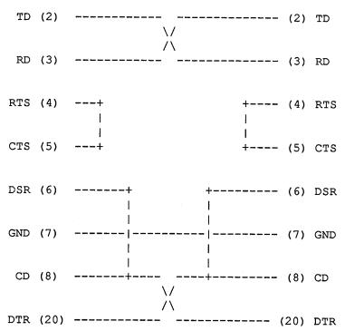
The above wiring generally eliminates concerns about ground loops between the computer and the peripheral. To do this use only Signal Ground, pin 7, and *not* Chassis Ground, pin 1.
