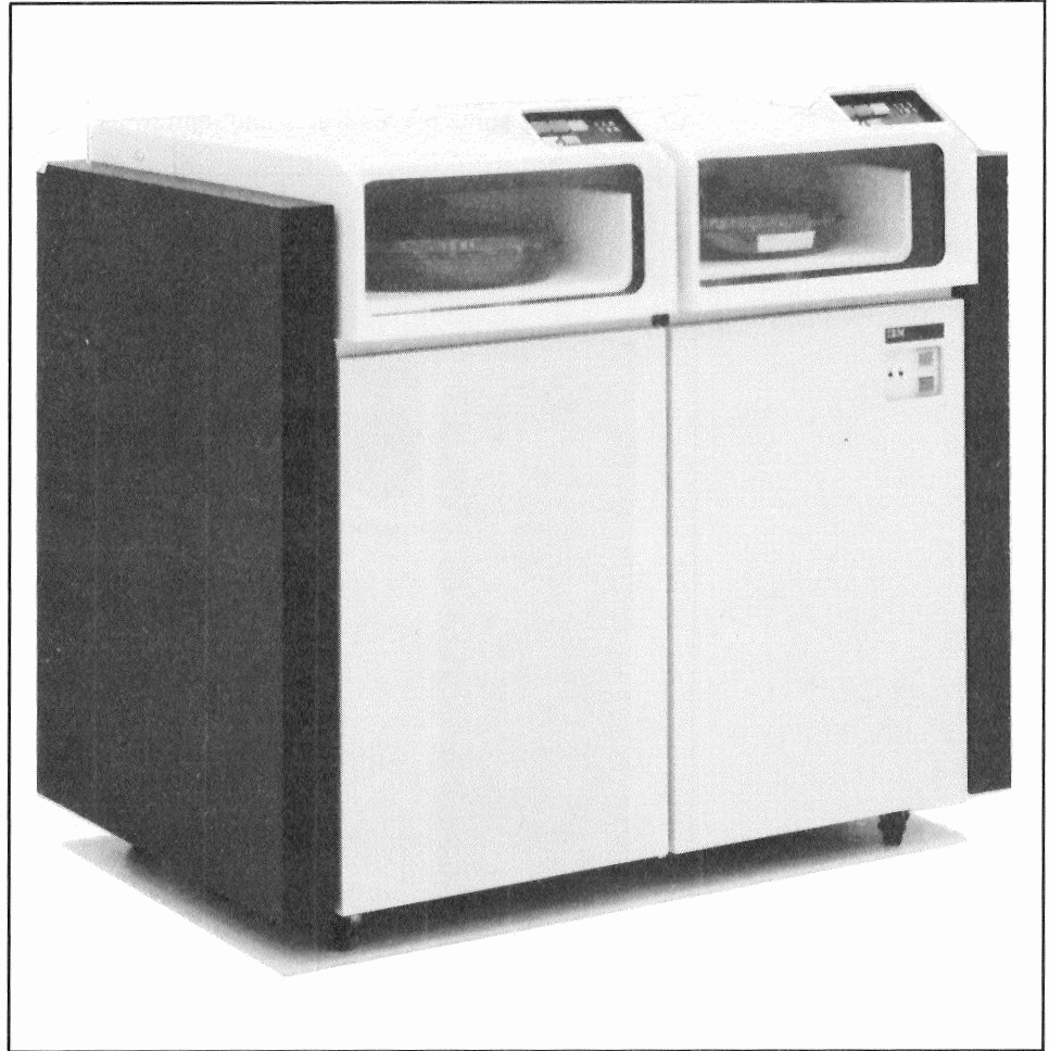
Figure 2-3340-1. 3340 Direct Access Storage Facility
