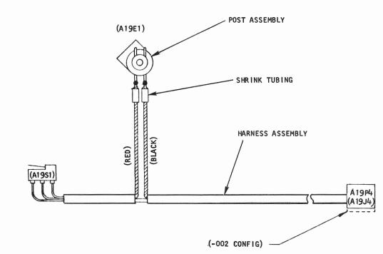
Figure 6. Band Interlock/Weld Sensor Assembly
