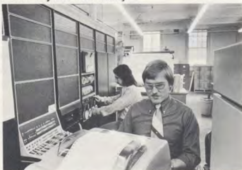
Ed DeJesus (left) checks the tape-drive of the REDAC PDP-15 computer system as Al Ackerman, group leader, inputs data on a Teletype.
