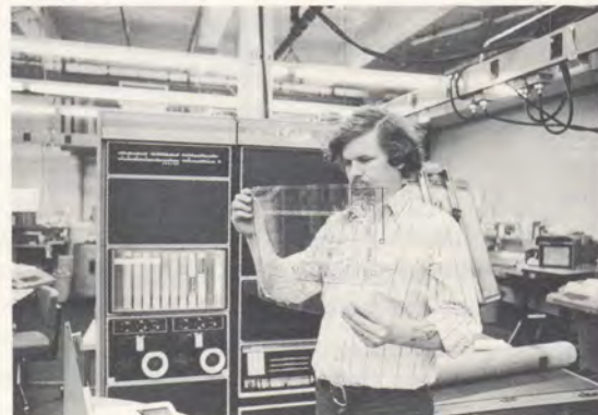
Gems Group Leader Al Brown examines a printed circuit board layout. This film was produced by the plotter and is the end result of the GEMS effort.
