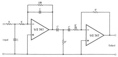
Fig. 5-27. Cascaded bandpass filter.
