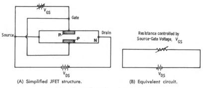
Fig. 2-11. Simple illustration of JFET operation.
