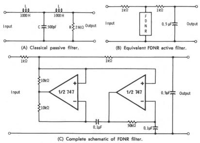
Fig. 5-23. FDNR low-pass filter with 320-Hz cutoff frequency.
