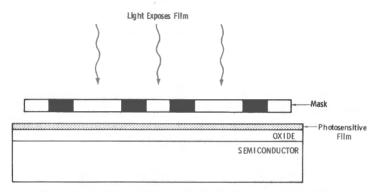
Fig. 2-15. Masking procedure for integrated-circuit fabrication.
