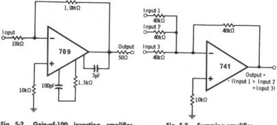
Fig. 5-2. Gain-of-100 inverting amplifier with external compensation.
