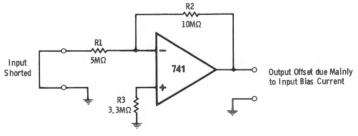
Fig. 4-7. Amplifier with gain of 2.
