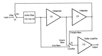
Fig. 7-6. Block diagram of function generator.
