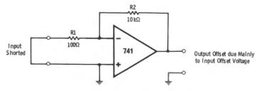
Fig. 4-6. Amplifier with gain of 100.
