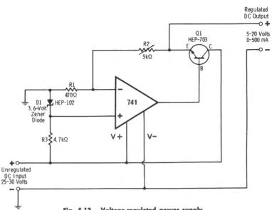
Fig. 5-13. Voltage-regulated power supply.
