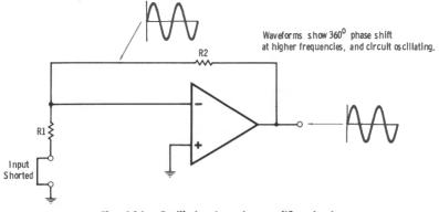
Fig. 4-14. Oscillating inverting-amplifier circuit.
