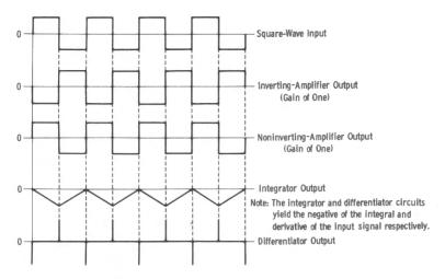
Fig. 1-10. Summary of output waveforms for a square-wave input.
