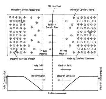
Fig. 2-6. Pictorial drawing of semiconductor diode, and plot of majoritycarrier concentration.
