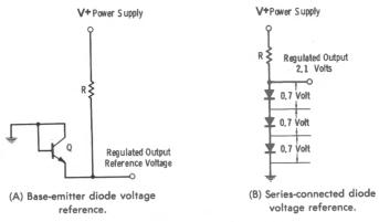
Fig. 3-3. Constant-voltage reference sources.
