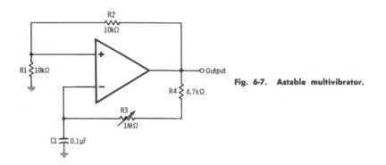
The frequency of the square wave depends on the values of C1, R3, and R4. Very low frequencies can be attained by using a large capacitance and large resistances. The high-frequency performance is limited by the slew rate of the particular op amp used.
