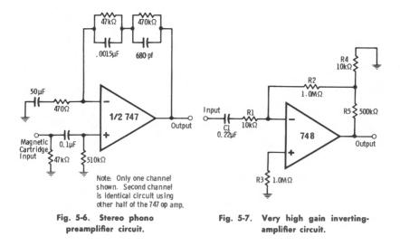
back resistance is that the circuit may have a large output offset due to input bias currents, as discussed in Chapter 4. Even when a resistor is used between the +input and ground, the input offset current may still cause a large output offset. The amplifier circuit shown in Fig. 5-7 avoids this problem by deriving its feedback signal from a voltage divider (R4, R5) across the op-amp output, rather than directly from the output. The gain of this circuit is given by:
