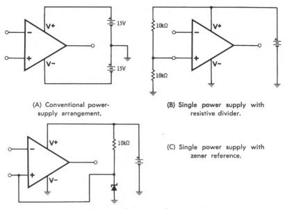
Fig. 4-19. Typical power-supply arrangements.
