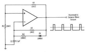
Fig. 6-9. Asymmetric square-wave generator.
