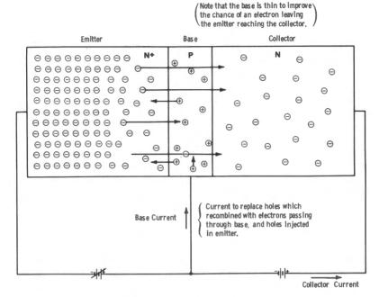
Fig. 2-10. Operation of the n + pn transistor.
