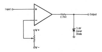
Fig. 6-3. Comparator with output limiter.
