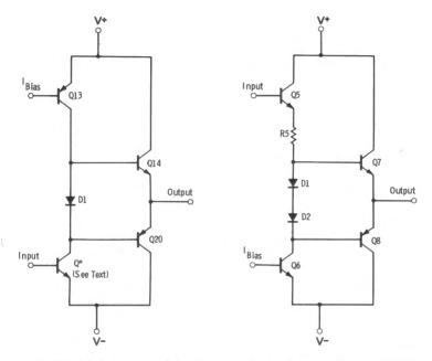
Fig. 3-14. Simplified schematic of the 741 op-amp level shifting/output stage.
