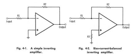
veloped across them. This voltage appears at the input of the op amp as a differential input signal because there is no corresponding voltage appearing at the other (grounded) input terminal of the IC. It is this differential input signal that is amplified by the op amp. The output offset voltage due to input bias current in this simple inverter circuit is approximately:
