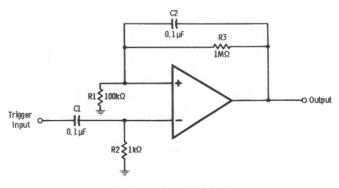
Fig. 6-6. Ac-coupled flip-flop.
