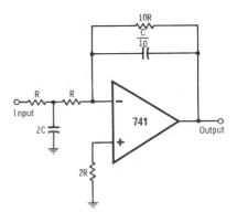
Fig. 5-21. Low-pass filter.
