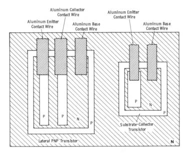
(B) Top view. Fig. 2-19. Monolithic pnp transistor structures.
