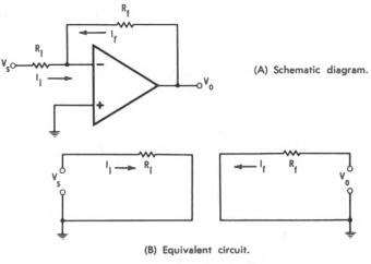
Fig. 1-5. Inverting amplifier.
