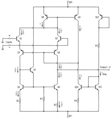
Fig. 3-12. Input stage of the 741 op amp with inputs grounded.
