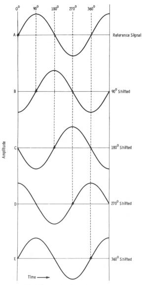
Fig. 4-11. Phase-shifted waveforms.
