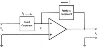
Fig. 1-2. Op-amp circuit with negative feedback.
