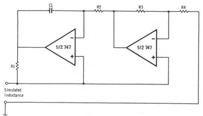
Fig. 5-18. Gyrator circuit.
