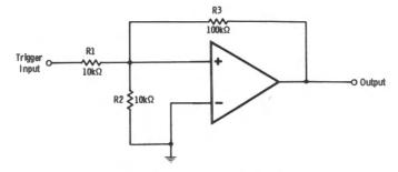
Fig. 6-5. Dc-coupled flip-flop.
