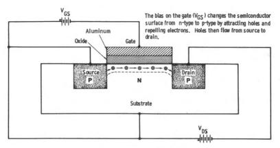
Fig. 2-13. Simple illustration of MOSFET operation.
