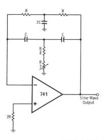
Fig. 5-17. Sine-wave oscillator.
