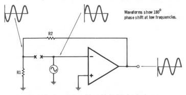
Fig. 4-13. Inverting amplifier with broken feedback path.
