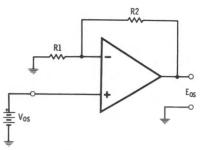
Fig. 4-5. Noninverting amplifier model for simple inverting or noninverting amplifier calculations.
