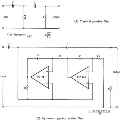
Fig. 5-25. High-pass filter using gyrator.
