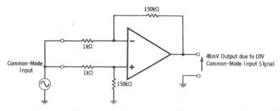
Fig. 4-18. Gain-of-150 differential-amplifier circuit with output due to common-mode input signal.
