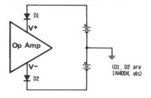
Fig. 4-21. Diodes D1 and D2 prevent opamp failure if power-supply polarity is reversed. tion. Two diodes, as shown in Fig. 4-21, can be used to prevent this type of failure.
