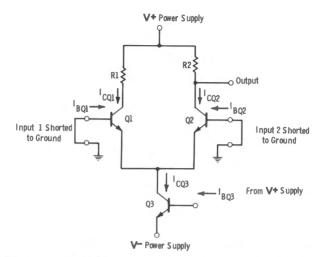
Fig. 3-4. A typical differential-amplifier circuit with inputs grounded.
