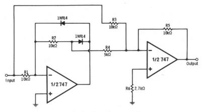
Fig. 5-11. Precision full-wave rectifier.
