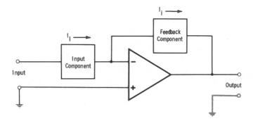
Fig. 1-3. Negative-feedback op-amp circuit with equivalent feedback current shown.
