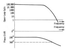
Fig. 4-12. Typical op-amp open-loop gain and phase shift as a function of frequency.
