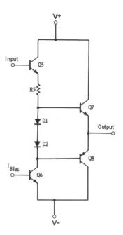
Fig. 3-9. A typical npn/pnp complementary output stage.
