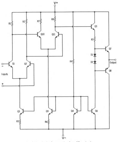
Fig. 3-10. A simple operational-amplifier circuit.
