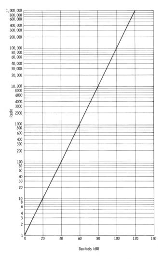
Fig. 4-16. CMRR ratio/dB conversion graph.
