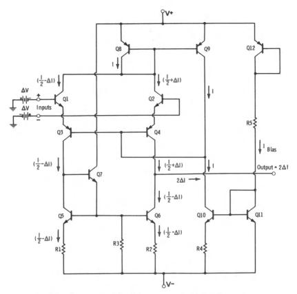
Fig. 3-13. Input stage of the 741 op amp with differential input signal.
