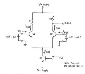
Fig. 3-5. A typical differential amplifier with a common-mode input signal.
