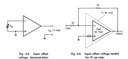
The input offset voltage may be modeled as a voltage source in series with the +input lead of an ideal op amp, as seen in the invertingamplifier circuit of Fig. 4-4. For this inverting-amplifier circuit, the output offset voltage due to the input offset voltage can be calculated as the response of a noninverting amplifier (Fig. 1-9A) to the input offset voltage, as shown in Fig. 4-5:
