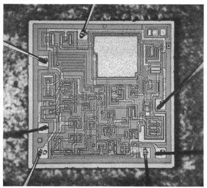
Courtesy Fairchild Semiconductor Fig. 2-16. A 741 op-amp chip with bonding wires attached.
