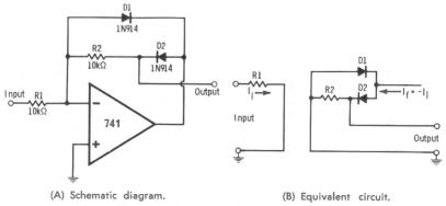
Fig. 5-10. Precision half-wave rectifier.
