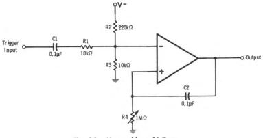
Fig. 6-8. Monostable multivibrator.
