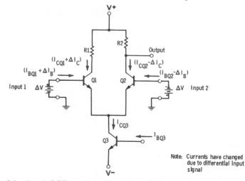
Fig. 3-6. A typical differential amplifier with a differential-mode input signal.
