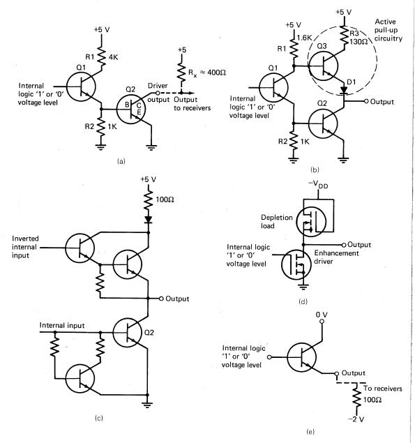
Figure 5-1 Typical driver circuits. (a) TTL open-collector. (b) TTL totem pole. (c) TTL tristate. (d) MOS. (e) ECL.
