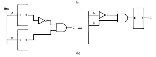
State reductions. (a) Redundant register elimination. (b) Pushing gates in Figure 6-5 front of registers.
