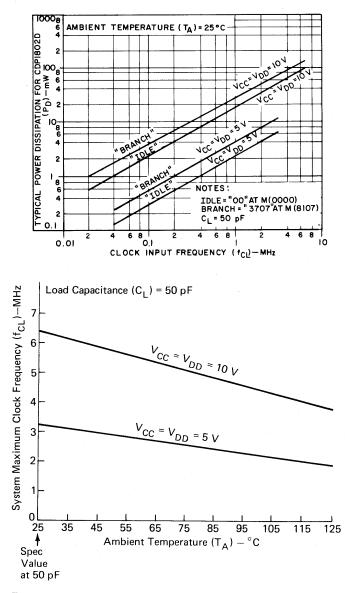
Typical power dissipation as a function of clock frequency for BRANCH instruction and IDLE instruction for CDP1802D.
