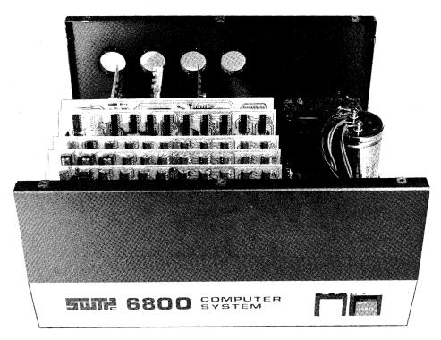
Figure 1-7 Southwest Technical Products' 6800-based personal computer system.
