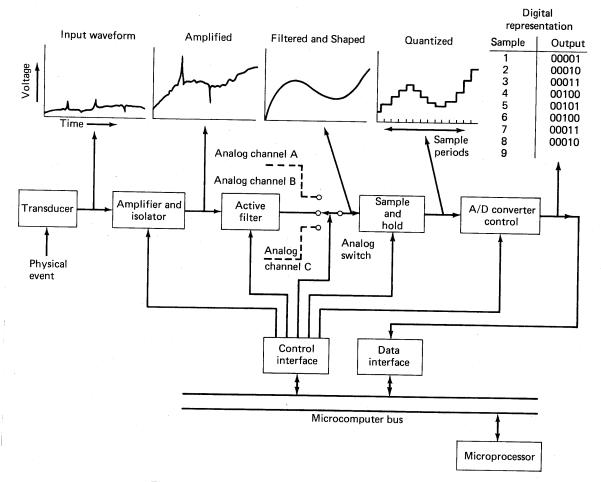
Figure 5-18 A microprocessor-based acquisition system.
