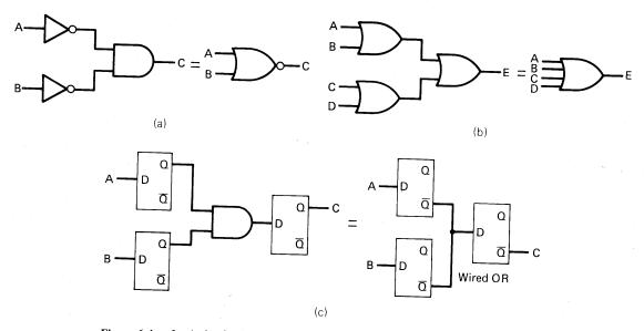
**Figure 6-4** Logical reductions. (a) Logical reductions by DeMorgan's law. (b) Consolidated gate reduction. (c) ECL gate reduction using wired-or approach.
