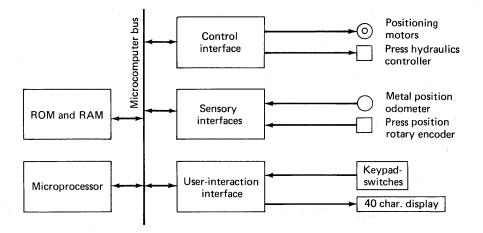
Figure 1-15 A microprocessor-based machine tool controller.
