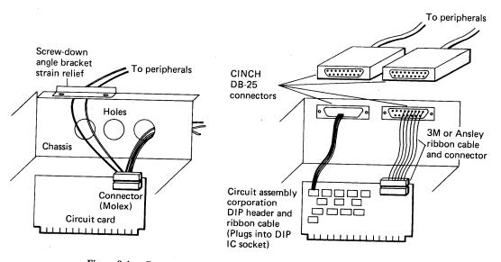
Figure 8-4 Connector systems. (a) Simple, inexpensive connector system. (b) Rugged, professional connector system.
