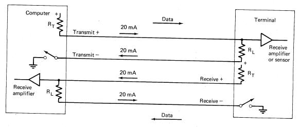
Figure 7-8 20 mA current-loop interface.
