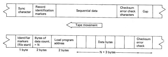
**Figure 3-16** Typical direct memory load tape formats. (a) Synchronous record format. (b) Direct memory load format (often used to load programs in microcomputer systems.)
