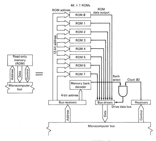
Figure 1-4 A typical microcomputer's ROM interfaces.
