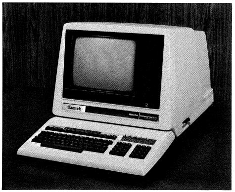
Figure 1-11 One of Ramtek's 6000-series intelligent graphics terminals. (Courtesy Ramtek Corporation.)
