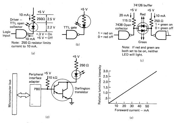
**Figure 5-25** LED driving methods and characteristics. (a) Standard LED with TTL driver. (b) LED with built-in resistor and TTL driver. (c) Red/green LED with dual current drive. (d) MOS device driving an LED. (e) Typical LED intensity curve.
