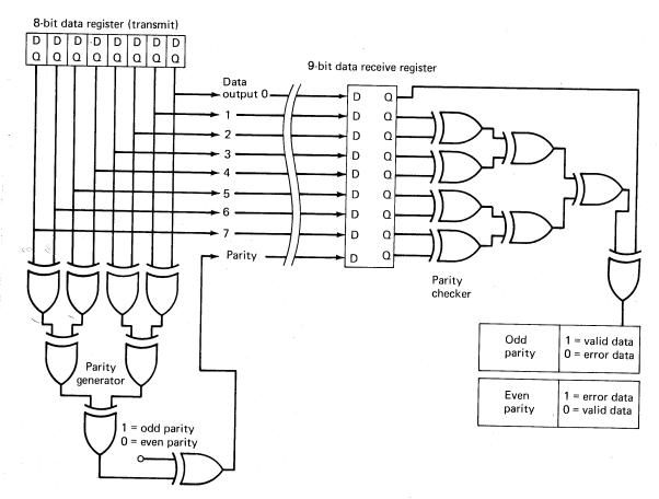
Figure 4-14 Parity generation and checking.
