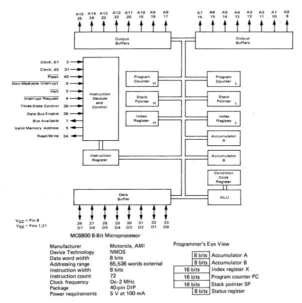
Figure 2-7 The Motorola M6800 microprocessor. (Courtesy Motorola Semiconductor Products, Phoenix, Arizona.)
