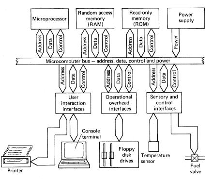
Figure 1-1 A typical microcomputer system and its interfaces.
