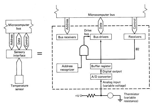
Figure 1-6 A typical microcomputer's sensory interface.
