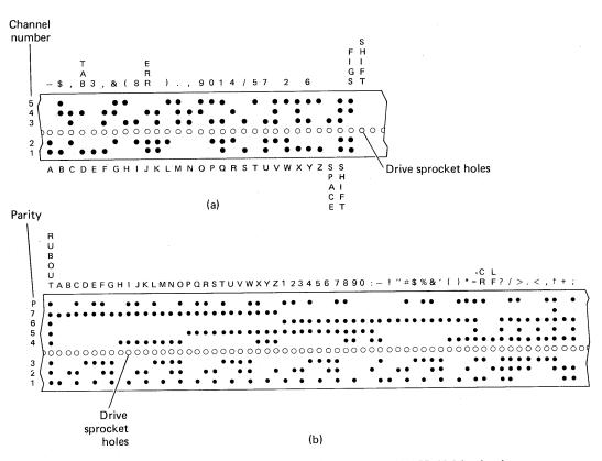
Figure 3-17 Paper tape formats. (a) 5-level code (29-code). (b) ASR-33 8-level code.
