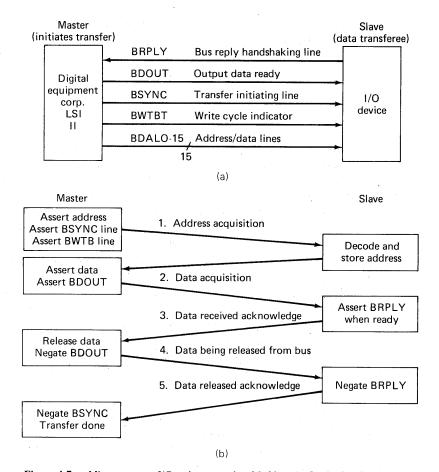
**Figure 4-7** Microcomputer I/O and memory handshaking. (a) Logic signals involved in a data output (DATO) cycle on the LSI 11. (b) Sequence of events in a DATO cycle.
