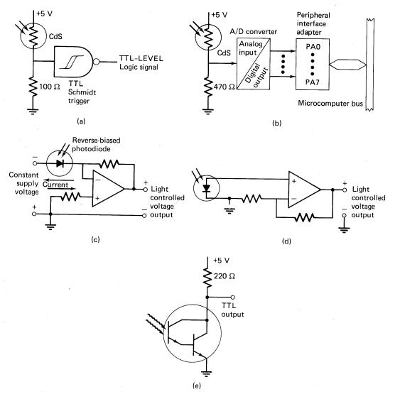
Figure 5-27Photoelectric circuits. (a) Simple on - off CdS photosensor. (b) Simplemicrocomputer-based light-level sensor. (c) Photodiode sensor (linear operation).(d) Photodiode sensor (logarithmetic operation). (e) Phototransistor (photodarlington)TTL-level light sensor.
