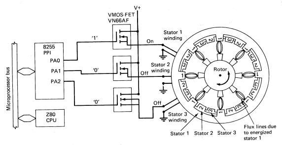
Figure 5-24 Microprocessor/VMOS/stepping-motor system.
