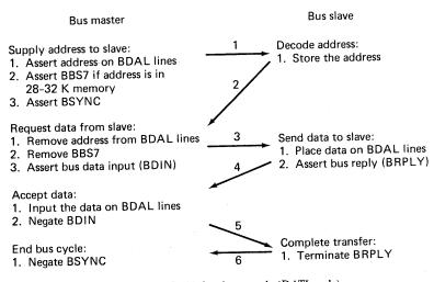
Figure 7-3 LSI-11 data input cycle (DATI cycle).
