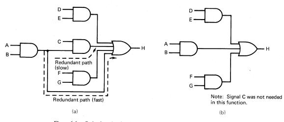
Figure 6-6Redundant signal paths. (a) Gating network with redundant signal path.(b) Equivalent, logically reduced gating network; no redundant paths exist.
