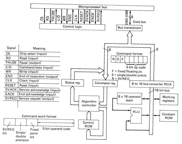
**Figure 5-16** The AM 9511 arithmetic processing unit (APU). (Copyright © 1978 Advanced Micro Devices, Inc. Reproduced with permission of copyright owner.)
