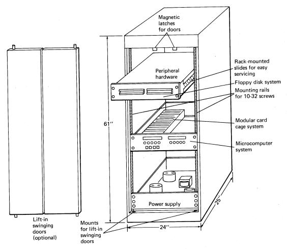
Figure 8-3 19-inch relay-rack mounting system.
