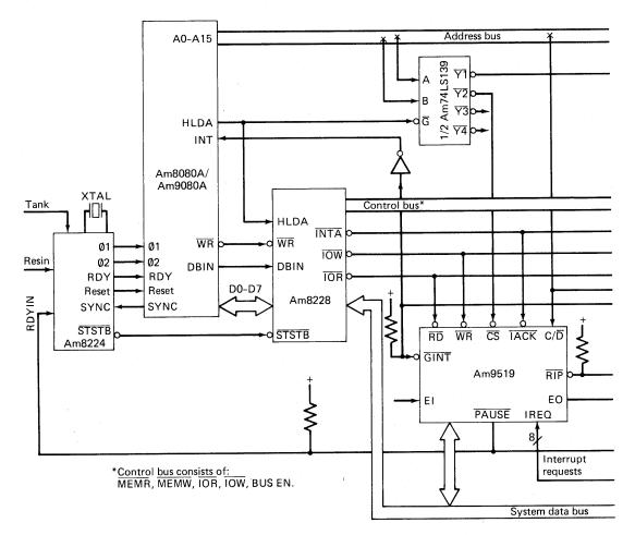
**Figure 4-10** A complete interrupt-driven I/O system based on the 8080. (Copyright © 1977 Advanced Micro Devices, Inc. Reproduced with permission of copyright owner.)
