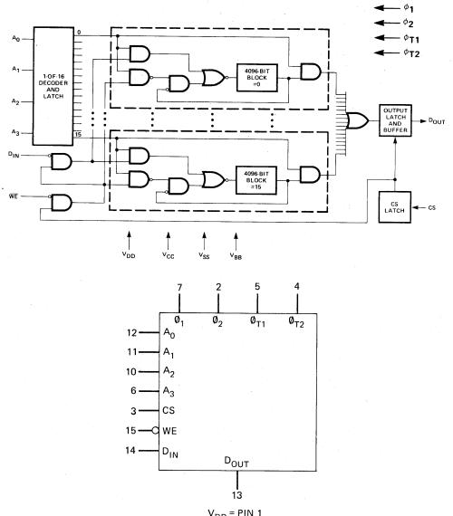
V<sub>DD</sub> = PIN 1 V<sub>CC</sub> = PIN 16 V<sub>SS</sub> = PIN 8 V<sub>BB</sub> = PIN 9
