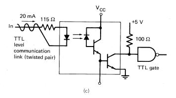
**Figure 5-28** Optoisolators. (a) Low-cost phototransistor isolator. (b) High-speed photodiode isolators. (c) Electrically isolated TTL communications receiver.
