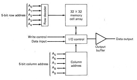
Figure 3-2 Memory peripheral circuitry and cells.
