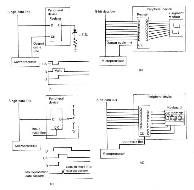
**Figure 4-4** Simple output and input data transfers. (a) Single-bit output transfer. (b) Parallel output transfer. (c) Single-bit input transfer. (d) Parallel input transfer.
