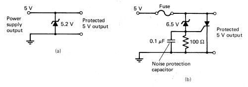
Figure 6-14 Overvoltage protection circuits. (a) Zener-diode voltage limiter. (b) SCR OVP "crowbar" fuse blower.
