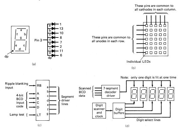
Figure 5-26 LED arrays and array drivers. (a) Common-anode 7-segment.
