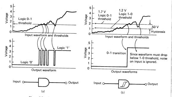
Figure 5-5 Transfer characteristics of standard versus Schmitt trigger gates. (a) Standard gate. (b) Schmitt trigger gate.
