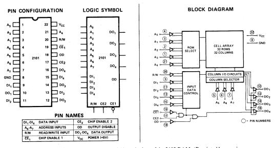
Figure 3-5 The 2101: a 256- by 4-bit equivalent of the 2102 RAM. (Reprinted by permission of Intel Corporation, Copyright 1976.)
