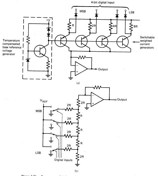
Figure 5-21 Two common digital-to-analog conversion methods. (a) Weighted-current-source D/A. (b) R-2R network D/A.
