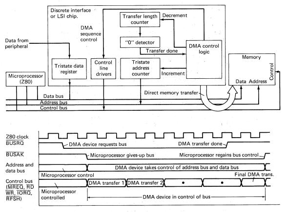
Figure 4-11 A typical microprocessor DMA cycle.
