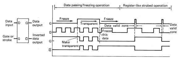
Figure 4-2 Bistable latch characteristics.
