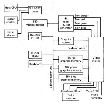
Figure 1-12 The Ramtek 6000 internal microcomputer bus. (Courtesy Ramtek Corporation.)
