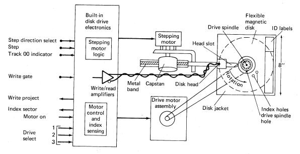
Figure 3-11 Details of a floppy disk drive.
