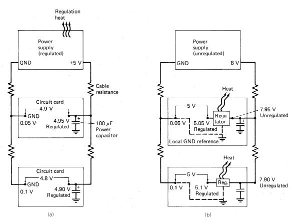
Figure 6-13 (a) Central and (b) onboard voltage regulation.
