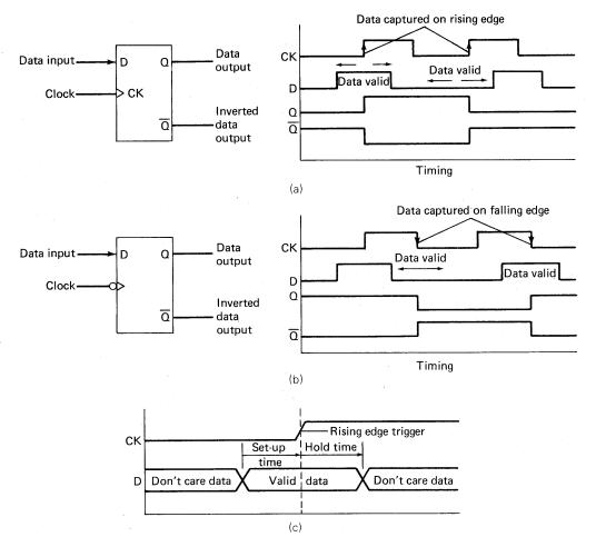
**Figure 4-1** Edge-triggered register characteristics. (a) Rising-edge-triggered register. (b) Falling-edge-triggered register. (c) Setup and hold times.
