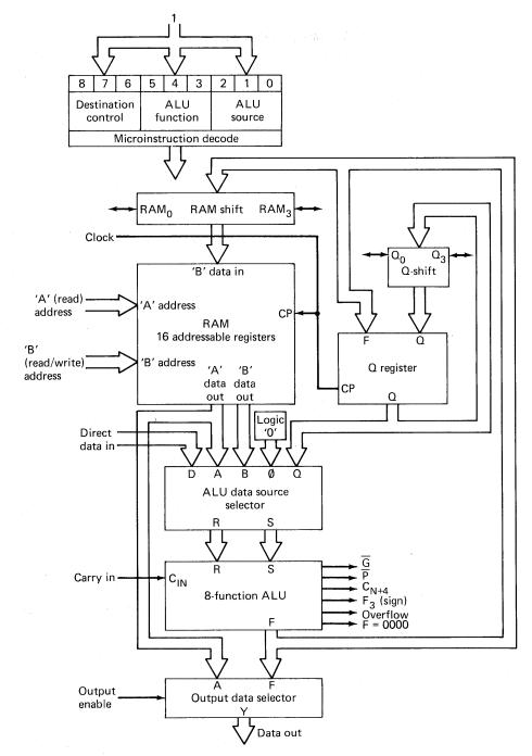
**Figure 2-17** Advanced Micro Devices' 2901 bipolar microprocessor slice. (Copyright © 1978 Advanced Micro Devices, Inc. Reproduced with permission of copyright owner.)
