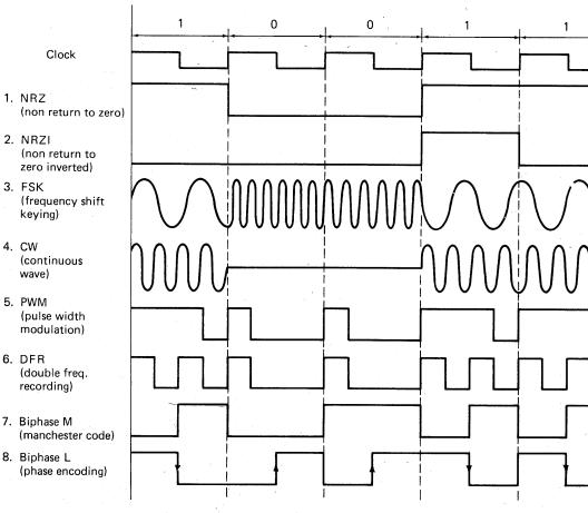
Figure 3-13 Common data recording and transmitting formats.
