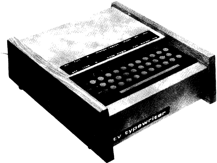
Fig. 1-1. The tvt-1 using TTL and shift-register memory.
