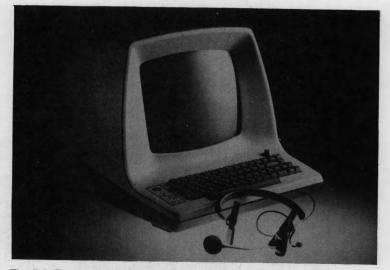
Fig. 5-6. The Heuristics 5000 converts the dumb terminal into a voice-entry terminal (courtesy of Lear Siegler Inc.).
