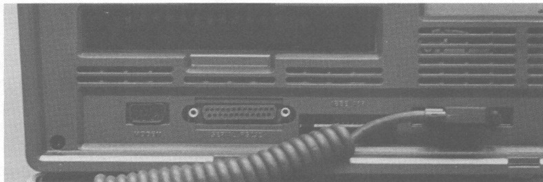
The six jacks and connectors for the Osborne computer.
