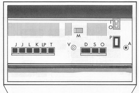
Figure 2.11. Connectors for external devices —
