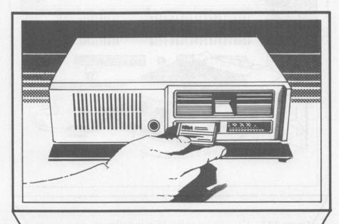
Figure 3.19. Inserting a PCjr cartridge
