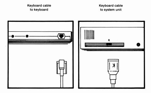
Figure 3.14. Keyboard cable connection
