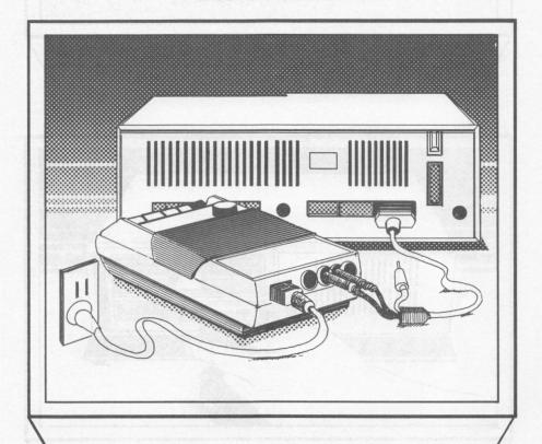
Figure 3.17. Cassette recorder/PCjr installation
