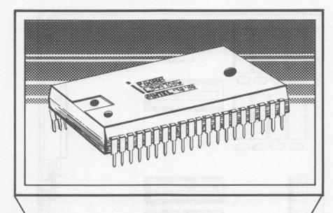
Figure 2.6. Intel 8088 microprocessor
