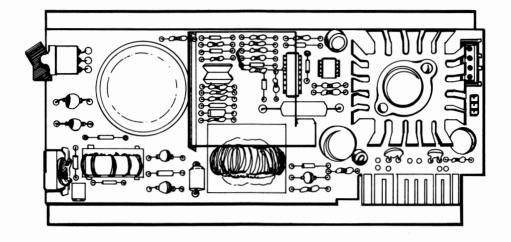
Figure 2.12. PCjr power supply board
