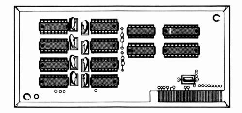
Figure 2.13. PCjr Memory and Display Expansion Board
