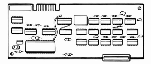
Figure 2.15. PCjr disk controller board
