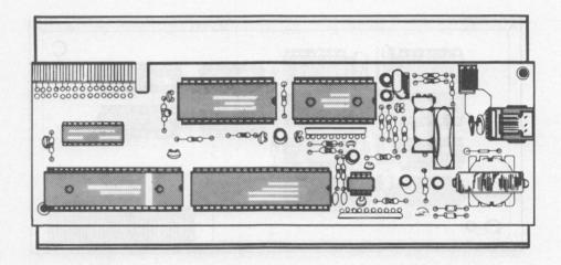
Figure 3.16. PCjr Internal Modem
