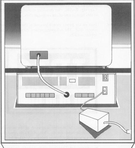
Figure 5.2. PCir system set-up (rear view)-
