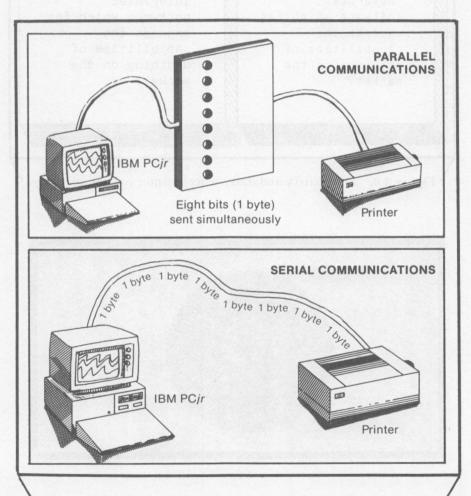
Figure 3.10. Serial and parallel communications
