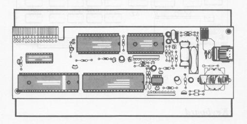
Figure 2.14. PCjr Internal Modem
