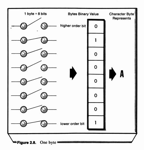
Most 8-bit microprocessors can only address (or work with) 65,536 bytes at any one time. Even though this number appears large, a 30 page document would fill this area. Most 16-bit microprocessors can address from 65,536 to 16 million bytes of memory. Moreover, 16-bit microprocessors process data at a speed from 2 to 10 times faster than 8-bit microprocessors.
