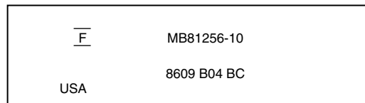
Figure 6.9 The markings on a typical older memory chip.
