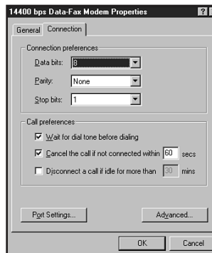
Figure 18.2 The Windows 9x control panel enables you to adjust the connection preferences for your modem.
