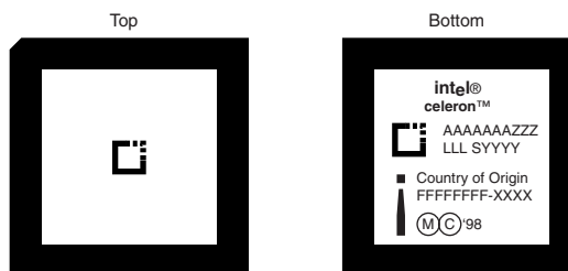
Figure 3.49 Celeron PPGA processor markings.
