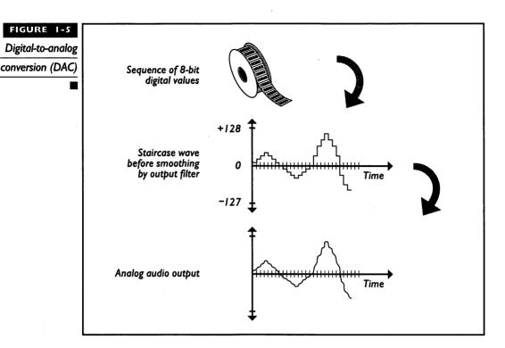
crete digital values representing the sound into a continuous analog signal by using a smoothing filter to round out the rough edges, as shown in Figure 1-5. Digital audio stored on disk is represented in Figure 1-5 by a tape reel with data bytes. The roughness of the reconstructed analog signal waveform has been exaggerated to emphasize the analog-to-digital conversion technique.
