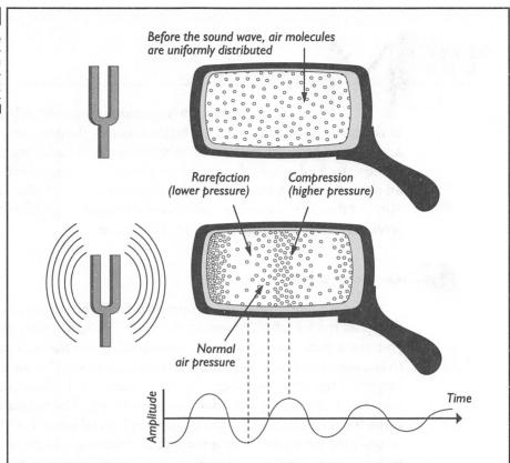
The frequency of sound is measured in units called hertz (Hz). A sound that vibrates once per second measures 1 Hz. Frequencies are often written in kilohertz (kHz), the unit representing 1,000 Hz. A young person with healthy ears can hear sounds in the range of 20 Hz to 20,000 Hz (20 kHz).
