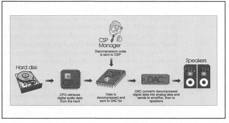
retrieved and sent to the CSP for processing. The CSP executes the program in its memory, decompresses the data, and sends it to the DAC. The DAC converts the decompressed digital data to analog data and hands it to the onboard amplifier, which in turn sends it to the speakers.
