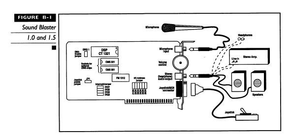
As shown in Figure B-1, the DSP chip is numbered CT 1321 on the 1.0/1.5 card and is the largest chip on the card. When a presentation program wants to play notes through the FM synthesizer, the DSP must accept the data from the computer and instruct the FM chip on how to play the music. When a game wants to surprise you with a digitally recorded explosion, the DSP accepts the sound data from the computer and converts it from digital to analog form so that you can hear the sound.
