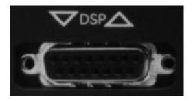
All NeXT computers include a digital signal processor (DSP) port providing direct input/output to the Motorola DSP56001 chip on the NeXT computer's CPU board. This port can accept digital input from laboratory equipment, analog-to-digital converters, or CD-quality audio devices. Several commercial suppliers offer external devices for analog-to-digital conversion and live sound, music or video input. Details on these products is found in the *Software and Peripherals Catalog*.
