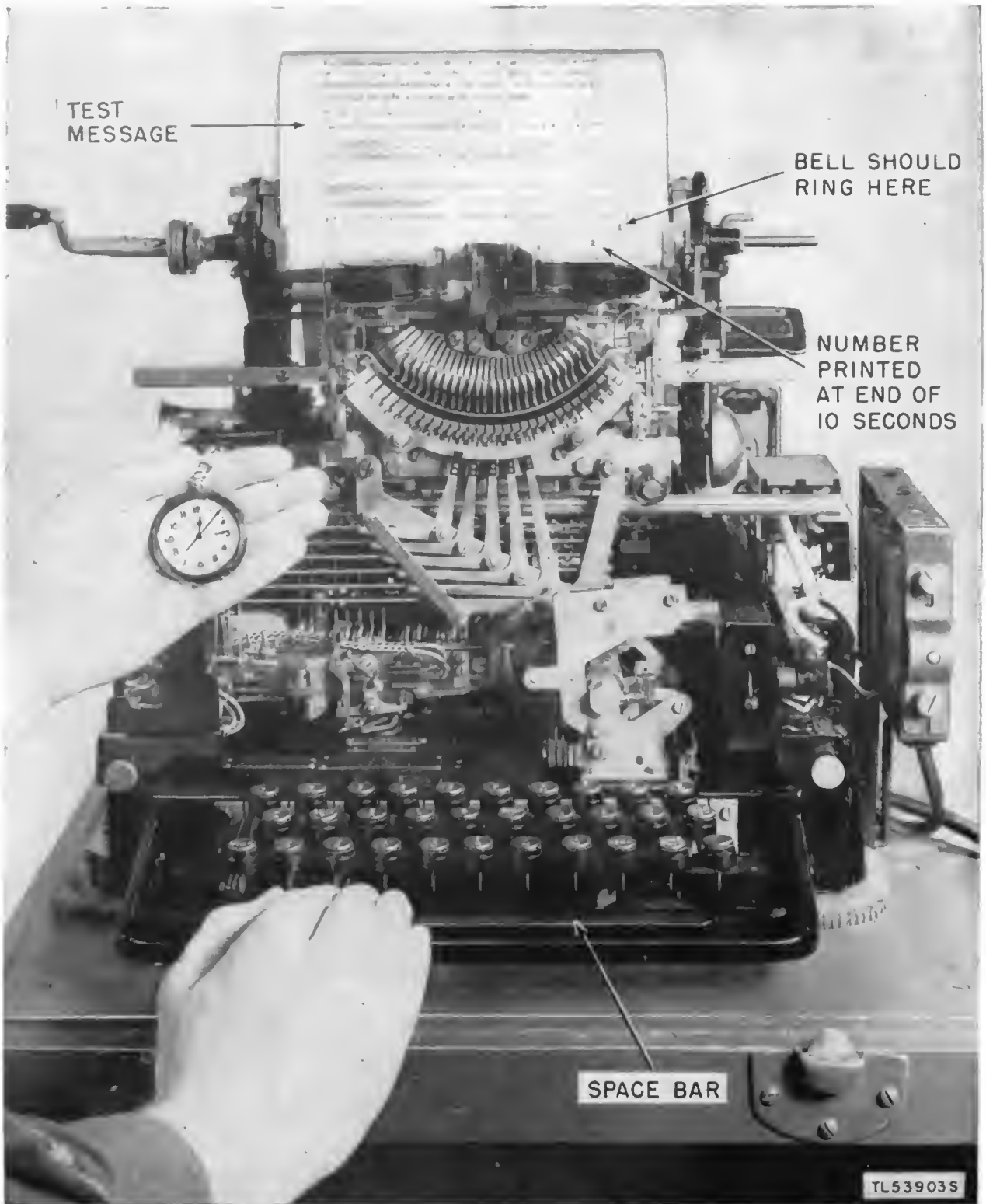
Figure 49. Checking motor speed by timing method.
