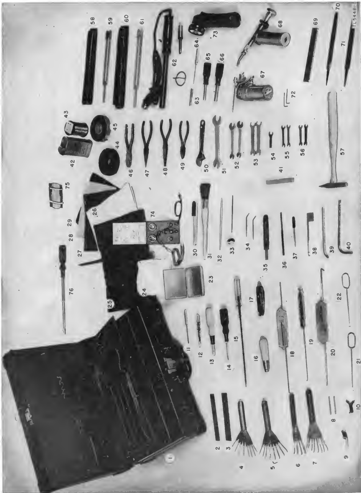
Figure 52. Tools and materials contained in Tool Equipment TE-50.
