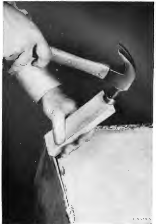
Figure 28. Opening metal container with wooden block.
