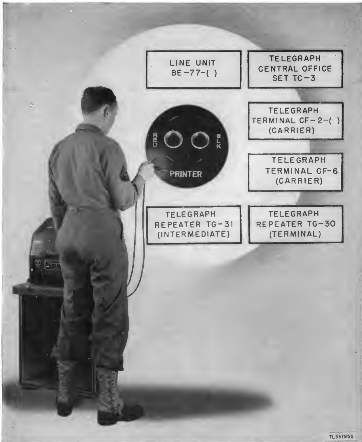
Figure 44. Typical jack connection to associated equipment.
