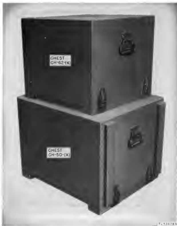
Figure 17. Complete teletypewriter packed for transportation and storage.
