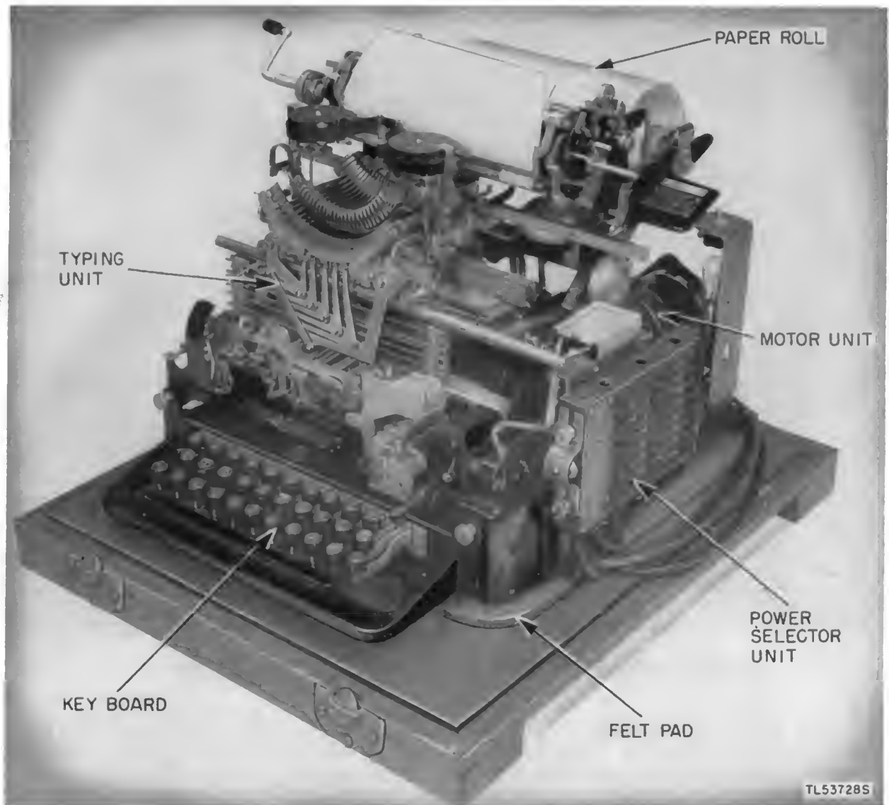
Figure 7. Teletypewriter TG-7-B base, keyboard, and typing unit assembled.
