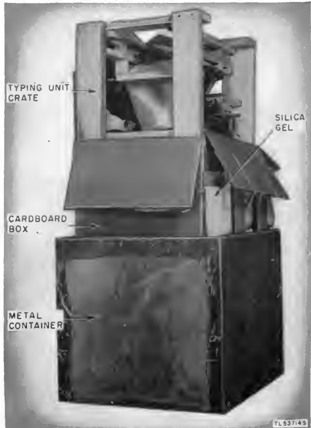
Figure 31. Removing typing unit from metal container.
