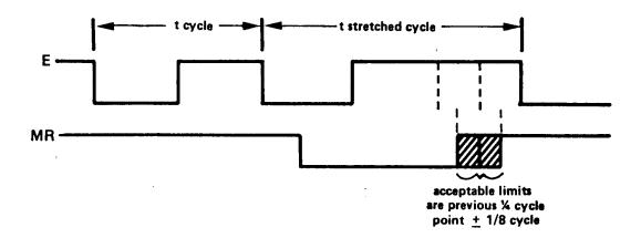
The following procedure can be used to measure the cycle stretches of the various SWTPC peripherals. Measurements require a good dual channel, triggered sweep, calibrated oscilloscope.
