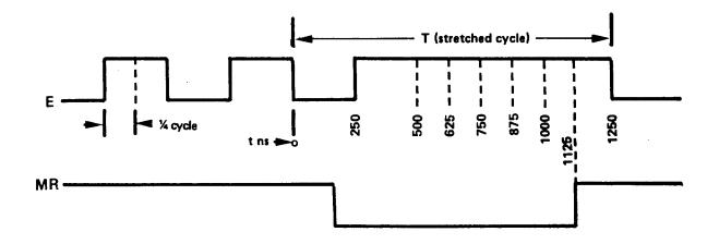
The cycle shown above has a T (stretched cycle)=1250 nS. Notice that MR goes high exactly one quarter cycle sooner, at 1125 nS. Timing diagrams for proper setup are shown below:
