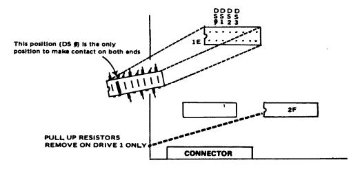
( ) On the other drive, bend straight out the pins of its jumper block as shown below. Re-install it as shown.
