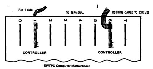
() Double check to be sure the cable is installed securely on the drives. All cables should be installed as in the following pictorial. By running the cable through the hole in the rear of the chassis the only natural way for the connectors to fit will be the right way, as shown. Be very careful that the cable is installed correctly--incorrect installation can cause damage to the controller and the drives.
