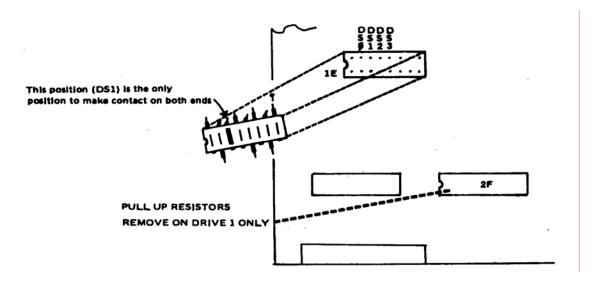
() Located on this drive below and to the right of the jumper block you will notice what appears to be an IC in a socket. This is an array of pull-up resistors and should be removed. This drive is now programmed as DRIVE 1.
