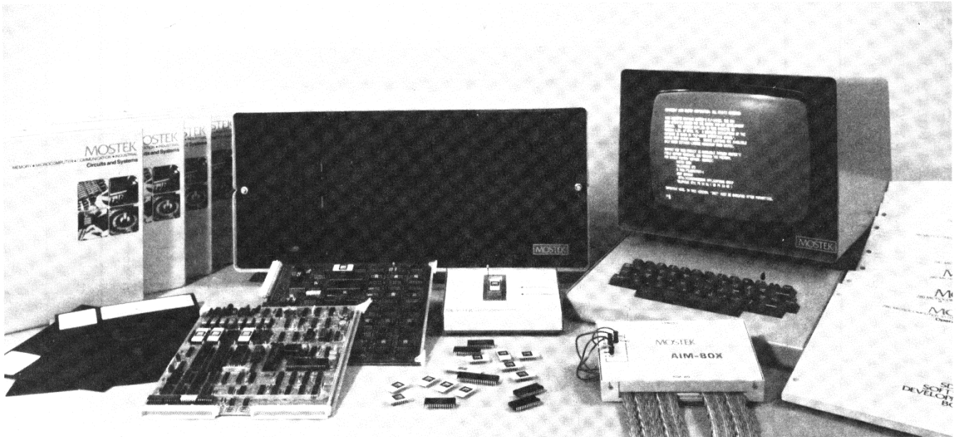
VIEW OF THE SYS-80FT DUAL FLOPPY DISK MICROCOMPUTER SYSTEM SHOWING ALSO OPTIONAL BOARDS AND ACCESSORIES
