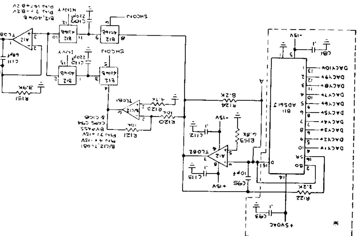
The circuitry within the dotted lines is optional circuitry for DAC 6012 at positions B11 and D11.
