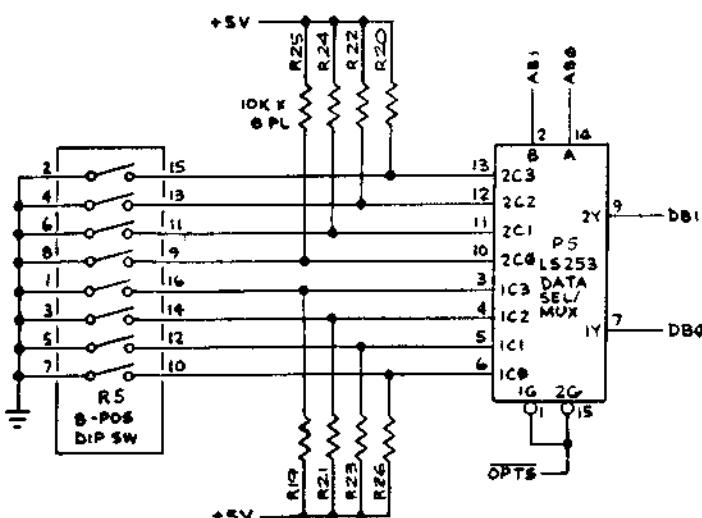
**The game option switches are read by the MPU when OPTS (option switch enable) is low. Switch toggles to be read are selected by AB0 and AB1 from the MPU. Switch toggles 1, 3, 5 and 7 are read on data line DB0 and toggles 2, 4, 6 and 8 are read on DB1. Toggle inputs are "on" when pulled to ground.**
