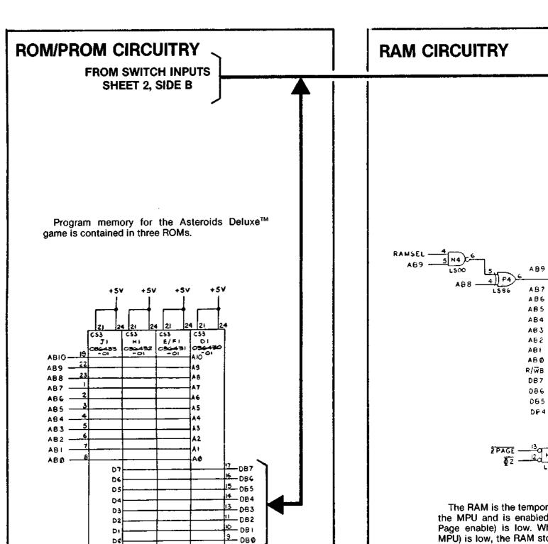
The RAM is the tempore the MPU and is enabled Page enable) is low. WI MPU) is low, the RAM stoput (DB0 thru DB7) at the by the MPU address bus (R/WB is high, the MPU rebyte at the addressed local
