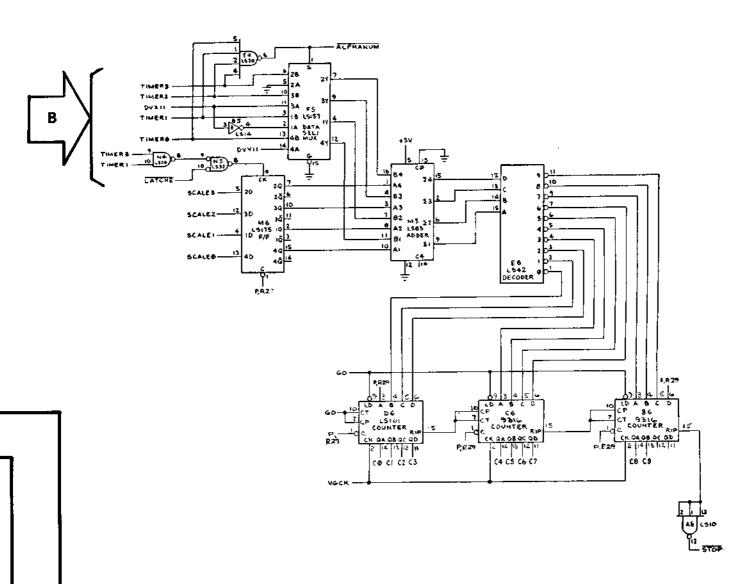
The purpose of the vector timer is to time out the length of time it takes to "draw" an actual vector on the monitor display. During the interval when the X- and Y-position counters are actually drawing the vector, STOP is high. This prevents the vector-generator state machine from advancing to its next state until the vector currently being drawn is completed. As soon as the vector has been drawn, STOP goes low, allowing the state machine to advance to the next state in its intended sequence.
