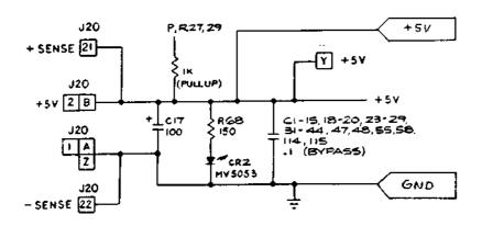
This circuitry consists of the PCB inputs and outputs for the +5 VDC logic power and 25 VAC input to the on board regulators. The +5 VDC inputs and outputs are discussed on Sheet 1, Side A of this schematic set.
