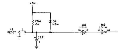
During inital power-up, the delayed charging of capacitor C22 causes a preset of flip-flop D3 and a clear of counter D4. This results in holding RESET input to the MPU low. When the charge of C22 reaches about 1.5 VDC, preset and clear inputs are removed. Counter D4 counts to 128 at 3-KHz rate, and RESET is removed (goes high) from the input of the MPU. This allows the logic power input to the PCB to stabilize before allowing the MPU to begin its initialization routine.
