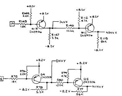
The x- and y-video inverter circuits are identical; therefore, only the x-video inverter circuit is explained. For invertered video operation, pin 19 is grounded which turns on transistor Q13 and turns off transistor Q12. In this state INV is  $\pm$  8.2 VDC and NONINV is  $\pm$  8.2 VDC.
