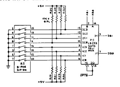
The game option switches are read by the MPU when OPTS (option switch enable) is low. Switch toggles to be read are selected by ABO and AB1 from the MPU. Switch toggles 1, 3, 5 and 7 are read on data line DBO and toggles 2, 4, 6 and 8 are read on DB1. Toggle inputs are "on" when pulled to ground.
