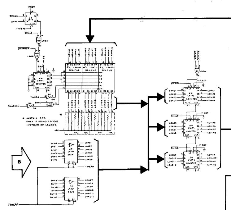
Counters F4, H4 and J4 contain the address of the next data byte (instruction) to be fetched from the Vector Generator memory. Because these counters point to the next instruction in memory to be retrieved and performed, they are called the program counter. This program counter is incremented one count (to the next sequential address) each time the information at its current address is loaded into data latch 0 or data latch 2.
