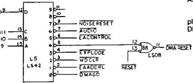
The address decoder performs the function of turning on or enabling the appropriate circuitry at the critical time, so that information can be transferred back and forth between the game circuitry and the MPU. The memory map below is for the Asteroids Deluxe™ game.
