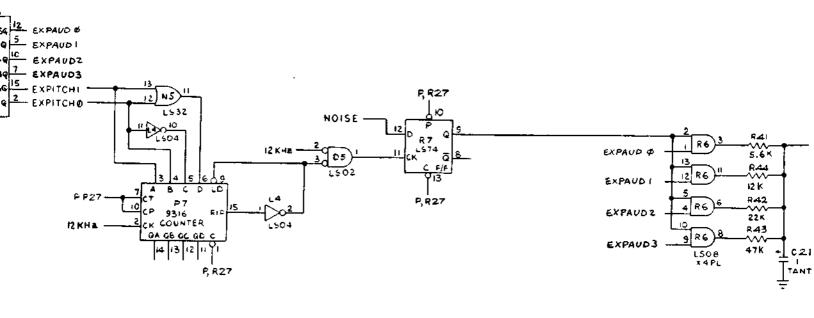
The EXPLODE sound is heard when any object explodes. Noise is sampled at a frequency determined by P7, and control bits EXPITCH0
