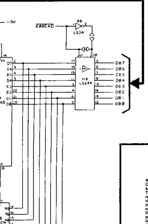
The High Score Memory circuit consists of an erasable reprogrammable ROM N9, latches L9, P9, N10 buffer M9, and timer N11.
