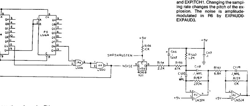
penerate random noise. This ed by P11 and produces the d heard when the ship is
