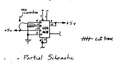
The SOL does not offer a baud rate of 134.5 baud. However, a simple modification can change the 110 baud rate to approximately 134.5 baud. The 110 baud clock is obtained by dividing the 1200 baud clock by 11 with a binary counter, U84. The counter can be made to divide by 9 if pin 12 is connected to a tieup instead of ground as in the SOL. This gives a baud rate of 133.33 which is within allowable tolerance limits. A partial schematic of the changes is given above.
