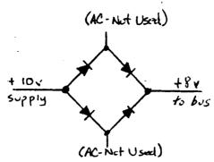
of the range specified in the manual. If the voltage is not brought down close to 8v. somehow, the on-board regulators overheat and will shorten the life of the board.
