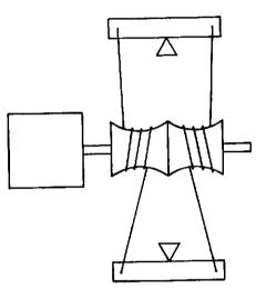
power of the motor is shared by various mechanisms as it's needed. So any particular mechanism can obtain as much energy as it needs up to the full capacity of the motor, while the average load on the main motor is comparatively low. The elements of the system are not much more complex than Tinkertoys, allowing the frustrated amateur to build his/her own experimental systems at a modest cost.
