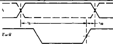
Fig. 3 Data Setup and Hold Time
