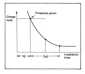
The irradiation energy for erasure of the MSM2716AS contents is  $15W \ sec/cm^2$ .
