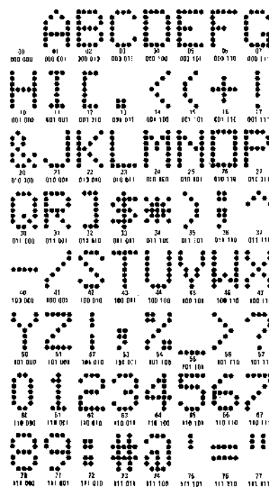
FIGURE 6. MM4240ABZ/MM5240ABZ Horizontal-Scan EBCDIC-8 Graphic Subset
