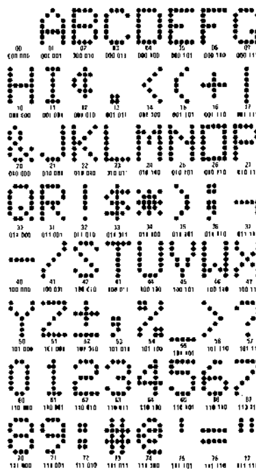
FIGURE 7. MM4240ACA/MM5240ACA Horizontal-Scan IBM EBCDIC Graphic Subset
