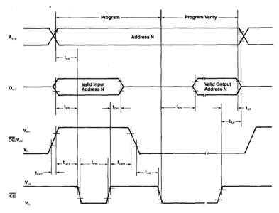
Note: ①  $0.1\mu\text{F}$  capacitor must be connected between  $\overline{\text{OE}}/\text{V}_{PP}$  and ground to suppress spurious voltage transients which may damage the device.
