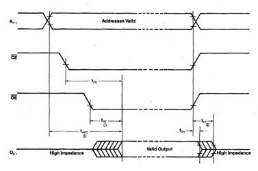
Notes: ①  $\overline{\text{OE}}$  may be delayed up to  $t_{\text{ACC}} - t_{\text{OE}}$  after the falling edge of  $\overline{\text{CE}}$  for read mode without impact on  $t_{\text{ACC}}$ . ②  $t_{\text{DF}}$  is specified from  $\overline{\text{OE}}$  or  $\overline{\text{CE}}$ , whichever occurs first.
