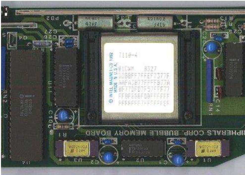
SILICONIX VQ7254CJ Drive Transistors on Intel Magnetics Bubble Memory Board
