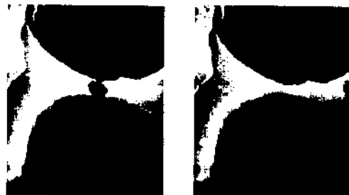
Figure 8. Blown and Unblown Polysilicon Fuse.
