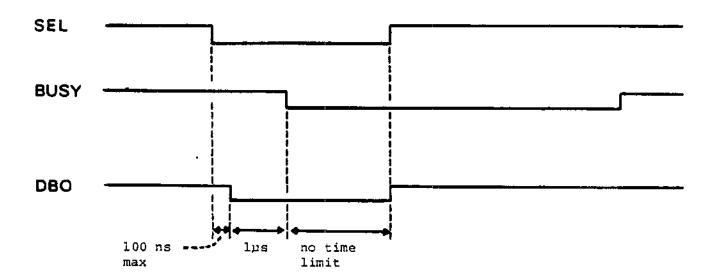
Note: SEL must be deasserted before the controller will assert REQ.
