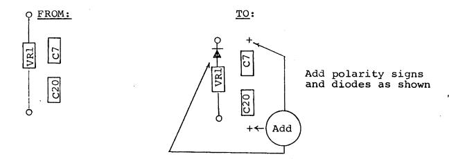
Change revision level of schematic and PCBA layout to Cl.
