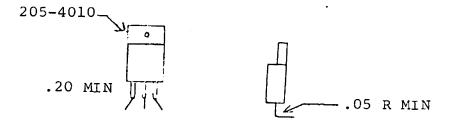
When mounting the 205-4010 triac to the process board, use the hardware configuration shown.
