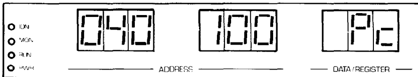
FRONT PANEL REGISTER DISPLAY (PROGRAM COUNTER SELECTED)
