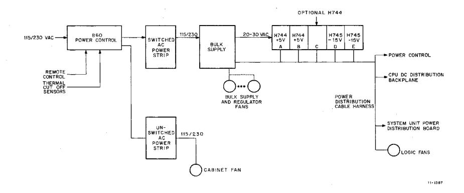
Figure 6-8 PDP-11/40 Power System Block Diagram
