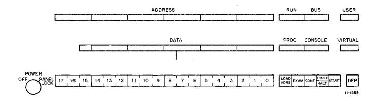
Figure 3-1 PDP-11/40 Programmer's Console
