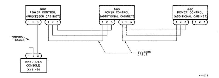
Figure 6.6 Power Control Interconnection
