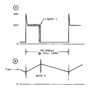
NOTE 1: 30 volt level shifts with AC input voltage. This value doubles in H746 (i.e. 60V). Small 120Hz jitter is normal
