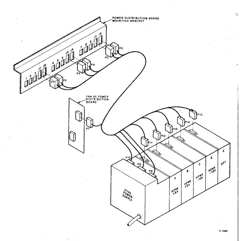
Figure 2-3 D.C. CABLE HARNESS 2-45A
