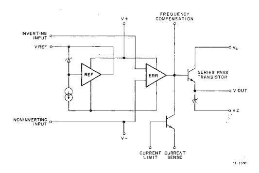
Figure 6-10 Simplified Diagram of Precision Voltage Regulator E1
