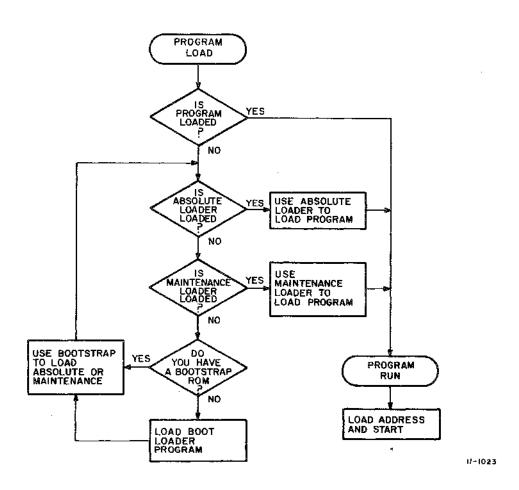
Figure 3-4 Flowchart of Procedure for Loading and Running Programs
