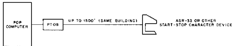
A. Local Terminal Connection
