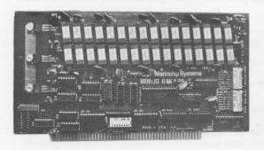
**64K RAM.** Our 64K RAM board provides 64K bytes of storage which operates in 16 bit mode, doubling system performance compared to 8 bit S-100 memories. The board includes programmable memory management hardware permitting bank selection in blocks of 4K bytes. Total system memory when using multiple 64K boards can be as large as 16 megabytes. Assembled: \$1050.
