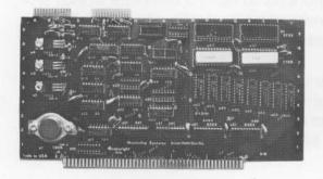
**PROM/RAM.** This board includes 2K bytes of PROM, 1K bytes of RAM, a serial I/O port with programmable baud rate, and programmable real time clock. The board provides room for up to 8K bytes of user PROM. This board is supplied with debug monitor and disc boot in PROM. Assembled: \$350, Kit: \$275.
