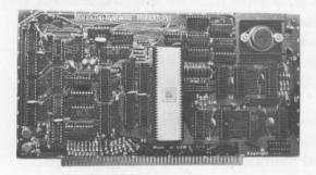
M9900 CPU. The processor board of the M9900 family. Includes TMS9900 16 bit processor with hardware multiply and divide, complete S-100 bus interface supporting both 8 and 16 bit memories, vectored interrupts, DMA, and both S-100 I/O and bitaddressable M9900 I/O. Assembled & tested: \$700, Kit: \$550. This price includes the basic software package (see below).
