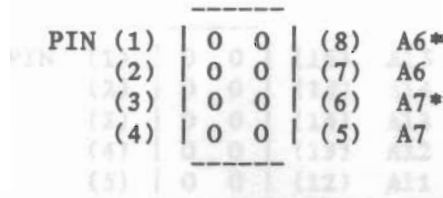
FIGURE 4.2 JUMPER CONNECTOR J-11 LOWER BYTE ADDRESS DEFINITION
