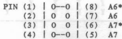
FIGURE 4.3 J-11 SAMPLE JUMPER CONFIGURATION FOR 80H/128D
