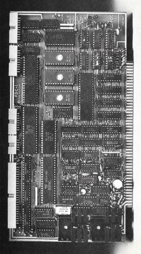
FDC-1 is a microcomputer on a board. It incorporates a monitor and all the I/0 normally required in a system.
