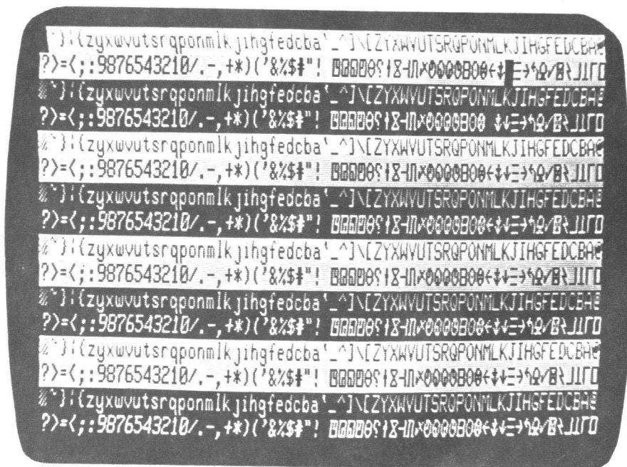
Figure 2-12. VDM-1 hardware-software test pattern (6574 character generator).
