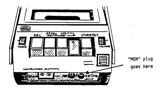
The cassette recorder is used to load BASIC and to save and load a BASIC program. The volume control should always be set at "8", and the tone control set at its highest setting, "+5". If the recorder is not powered by batteries, they should be removed. Whenever the recorder is used, the cable marked "MON" should be connected to the jack input labeled "ext. sp.".
